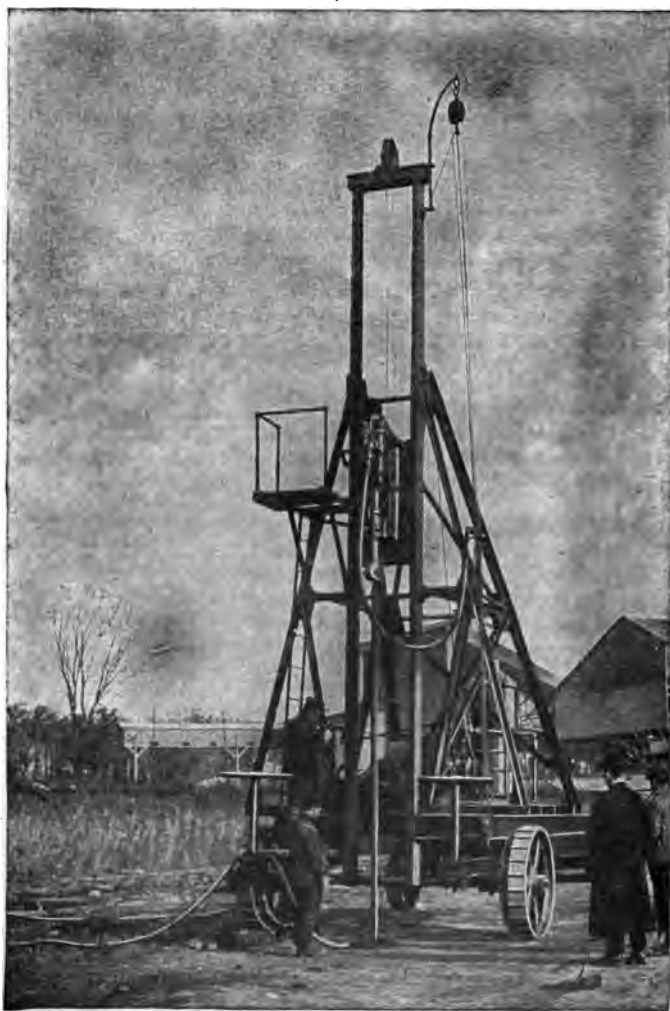
Fig. 36. Auto Traction Rock-Drill Capable of Drilling 5-in. Holes to a Depth of 50 Ft.
